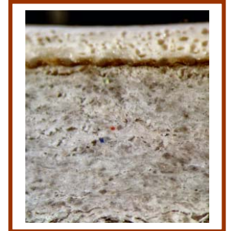
This belt is made from coated bonded leather fibre – it certainly is not leather!
